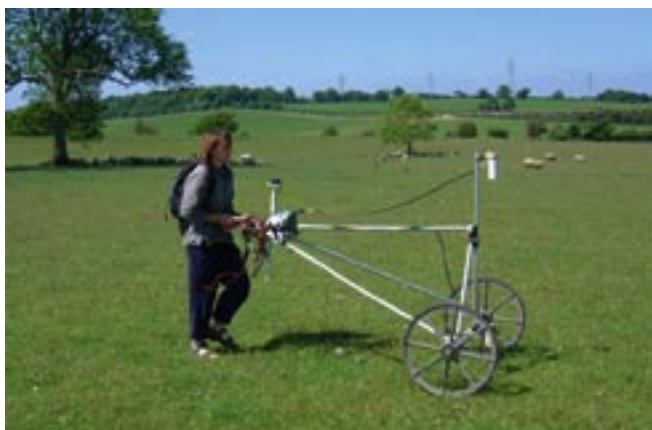
The caesium vapour magnetometer in use on site during the trial run in July. A satellite positioning system on the carriage records the location of each reading. Photo Will Bowden
